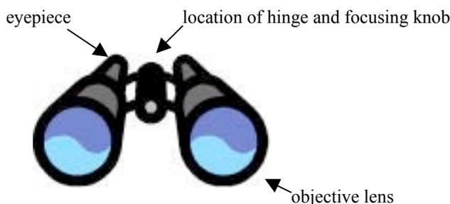
2. Find the side of the binoculars, right or left, with the adjustable eyepiece. Close the opposite eye, i.e. if the adjustable eyepiece is on the side that the right eye looks into then close the left eye. While looking through the binoculars, adjust the focus for the open eye until the image that the user is viewing is in focus. Use the main focusing wheel, usually on the top of the binoculars near the hinge, to bring the view into focus as the user looks through the eyepiece.
